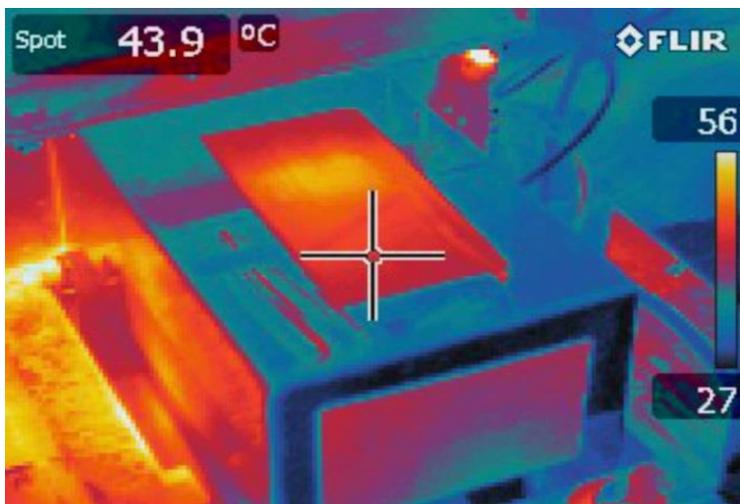
Following the installation of the heating elements within the calibration tile housing, the whole system and its output became extremely stable. At this point further development was not required to deliver the initial project aim of using the system output to manage the wash water operation on the four individual white centrifuges.
