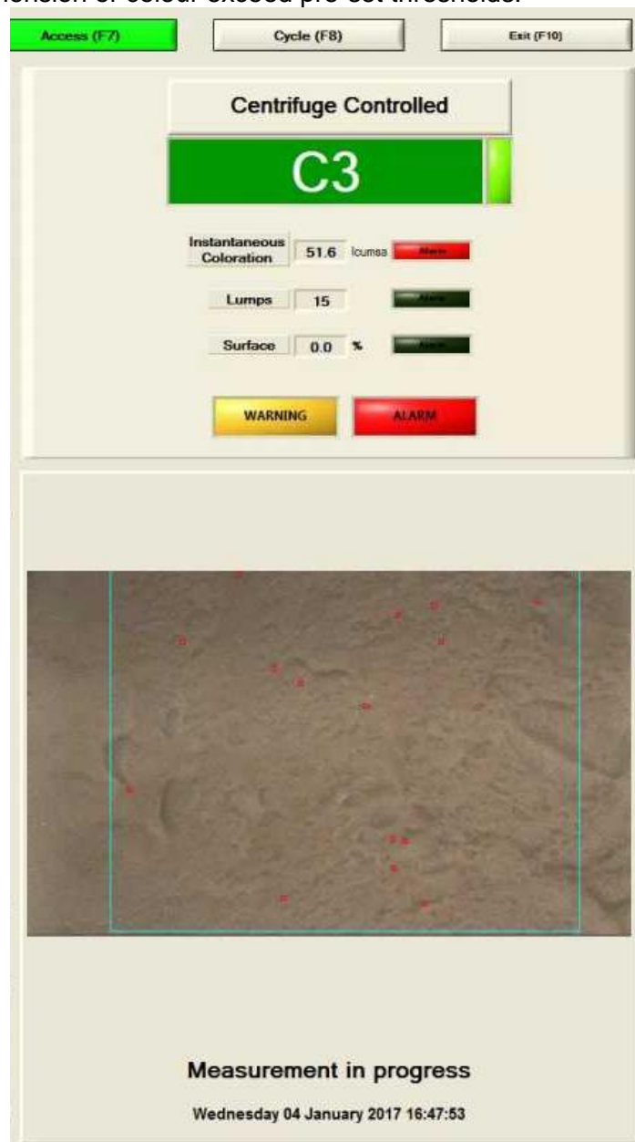
Figure 7: Very small brown lumps detection highlighted in red on the video
